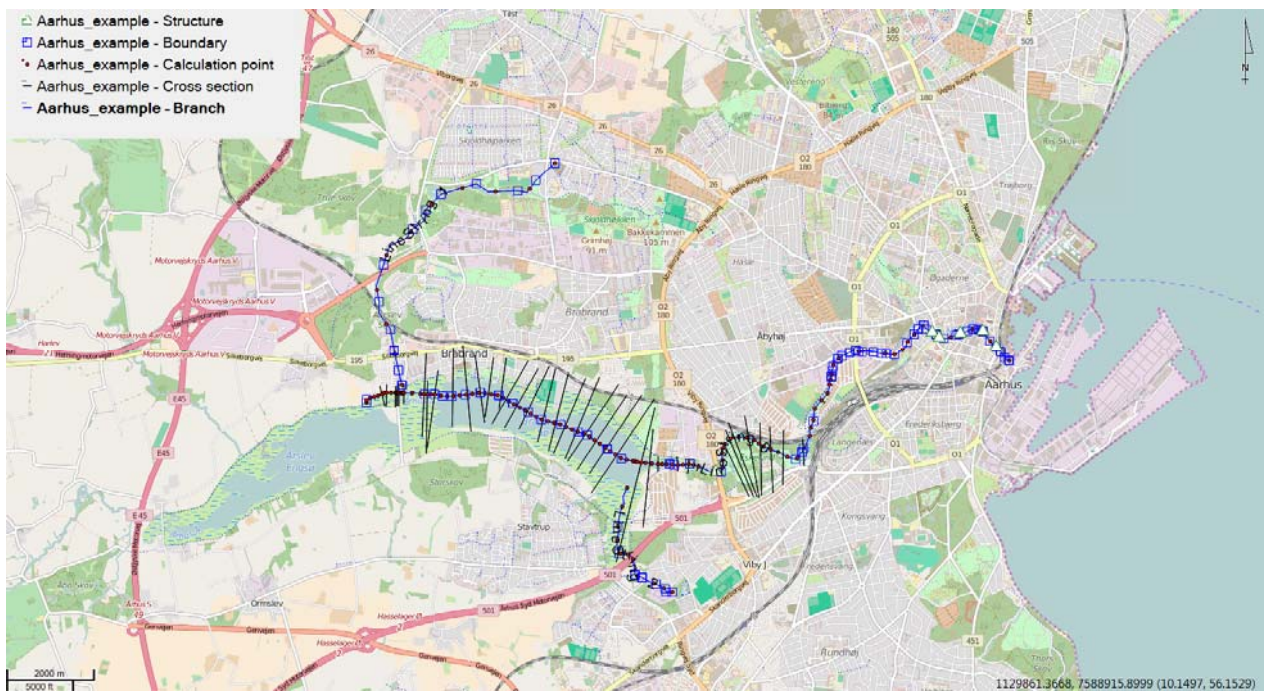
Figure 6 Schematic of MIKE 11/ECOLAB representation of Lake Brabrand and the Aarhus River
